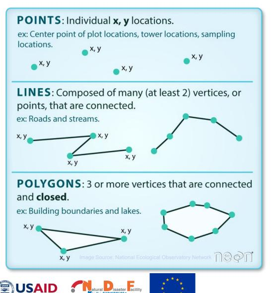
Vector data (point, line or polygon) are all made up of series of points or vertices
